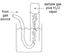
In today's experiment you will be collecting the gas from a regular cigarette lighter. After collecting it, you will make careful measurements of its mass, volume, temperature, and pressure. This will allow you to calculate the number of moles of gas trapped in the cylinder, which, along with the mass, will provide you with an experimental molar mass for the gas.
