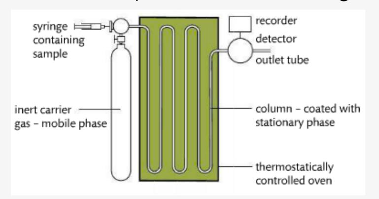
each component passes the detector, and time eluted is recorded - known as retention time
